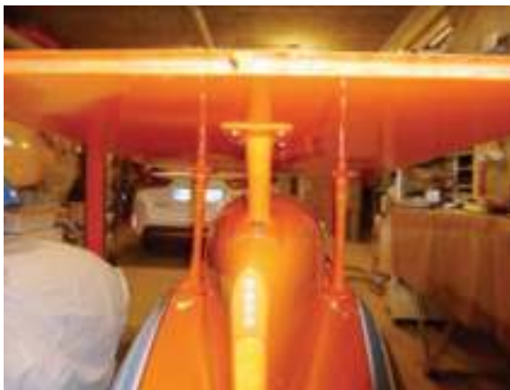
The panel can be tilted to capture the best sunlight.
