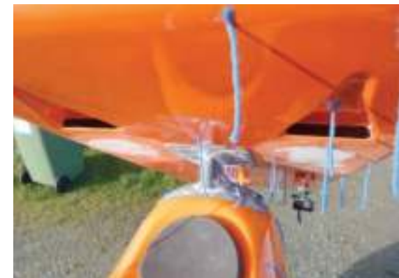
The woolen threads are used to visualize air flows.
