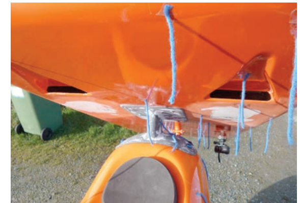
The woolen threads are used to visualize air flows.
